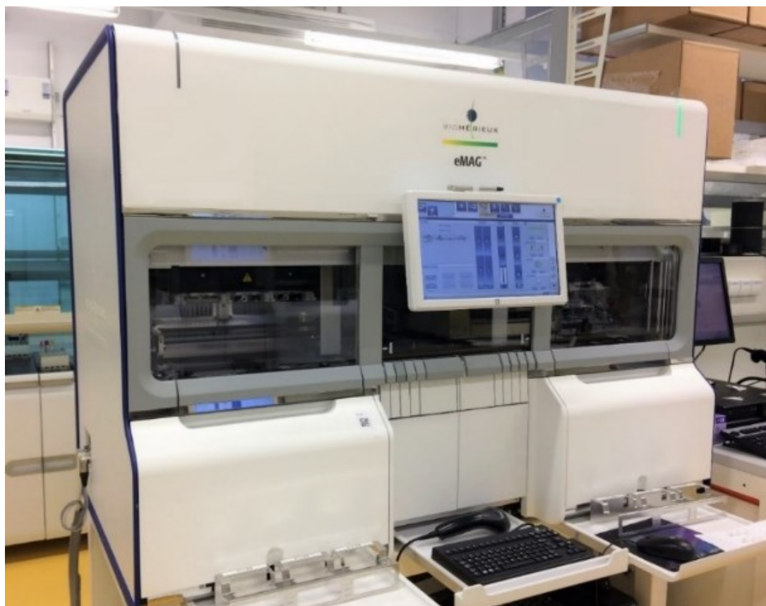
Figure 7: EMAG ® nucleic acid extraction platform (picture taken by Alexandra Radler on April 5, 2019).
