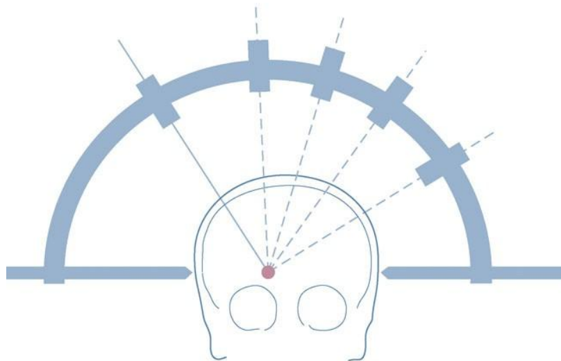
Figure 1. The Leksell arc-centered design with adjustable carrier. (9)
