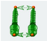
Figure 21: Interscrew distance measured at head and tip levels
