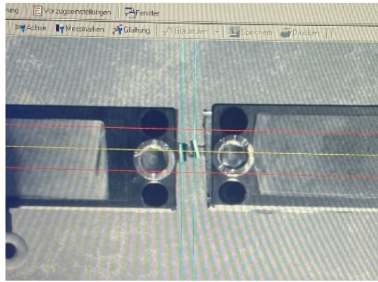
Figure 10: WinextNG (Videoextensometer ME46 NG, Messphysik Materials Testing GmbH, Fürstenfeld, Austria).
