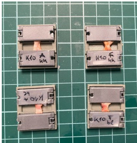
Figure 7: Samples shaped into dog-bone with 3D clamps.
