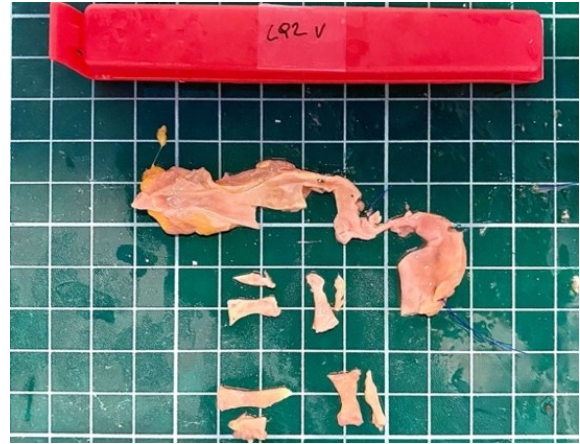
Figure 11: Dumbbell-shaped tissue samples of the attached gingiva and lining mucosa in the orientation "mc" and "bp"
