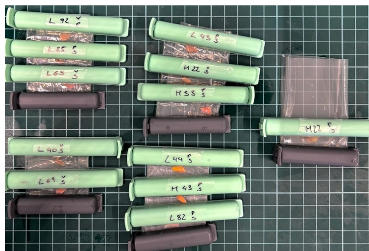
Figure 4: Samples in dialysis membranes divided by clips prior to submersion into the PEG solutions
