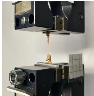
Figure 16: Sample torn by the tensile test, clamped in the uniaxial testing machine
