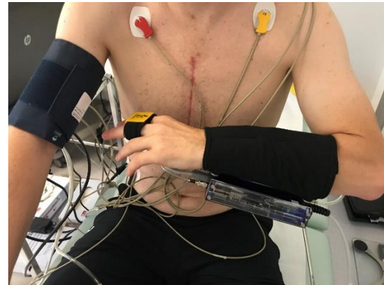
Figure 21 (left): image shows the 4 ECG electrodes and the 3 impedance electrodes placed on the chest. Reproduced from: Task Force Monitor Technical Specifications, CNSsystems, 04.2019.
