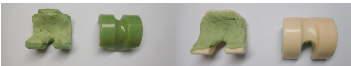
Figure 9-5: Femoral knee spacers covered with Palacos R on the non-articulating surface Legend: Left = Spacer A; Right = Spacer B
