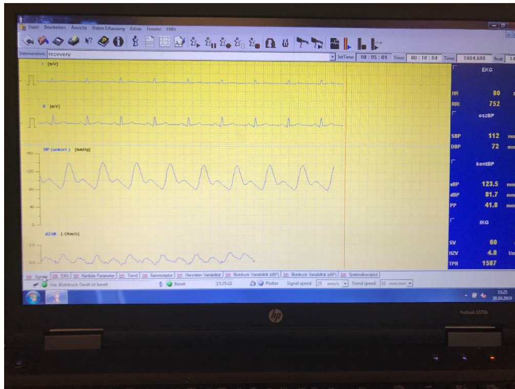
Figure 10: the “Signale”-screen of the TFM during a measurement. Showing from top to bottom the first and the second ECG derivation, the blood pressure curve of the arm oscillometer and the blood pressure curve of the finger plethysmograph below. In the blue box on the right the current values of HR, RRI, sBP, dBP, SV, CO and TPR are shown.
