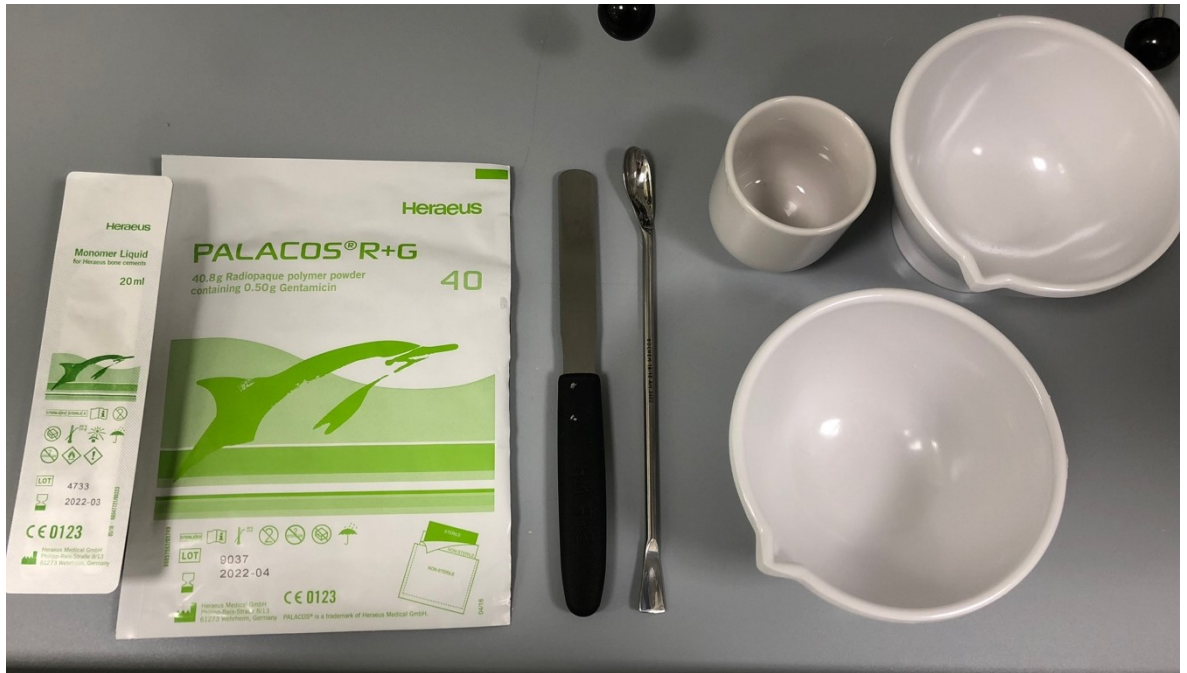
Figure 24: Experimental setup for producing cement bodies: from left to right: monomer liquid, polymer powder, spatula, spoon, ceramic bowl and two plastic bowls
