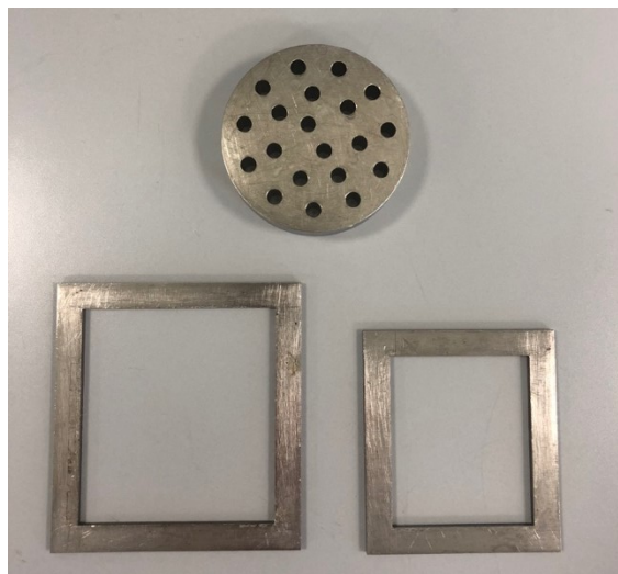
Figure 25: Molds for preparing cement bodies for mechanical testing
