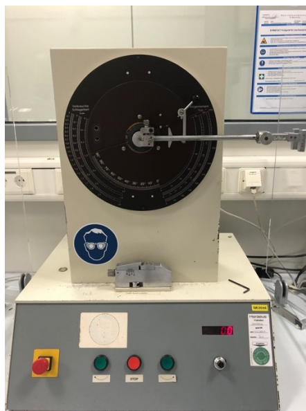
Figure 26: Starting position of Dynstat impact strength test
