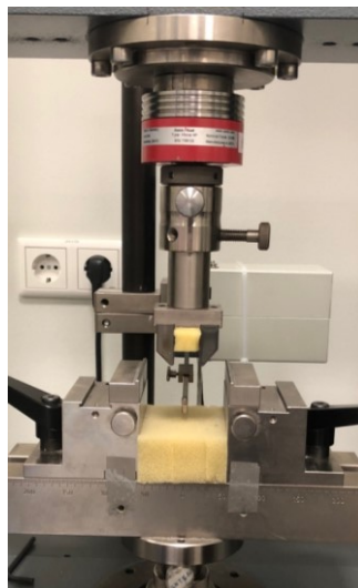
Figure 35: Starting position of four-point bending test
