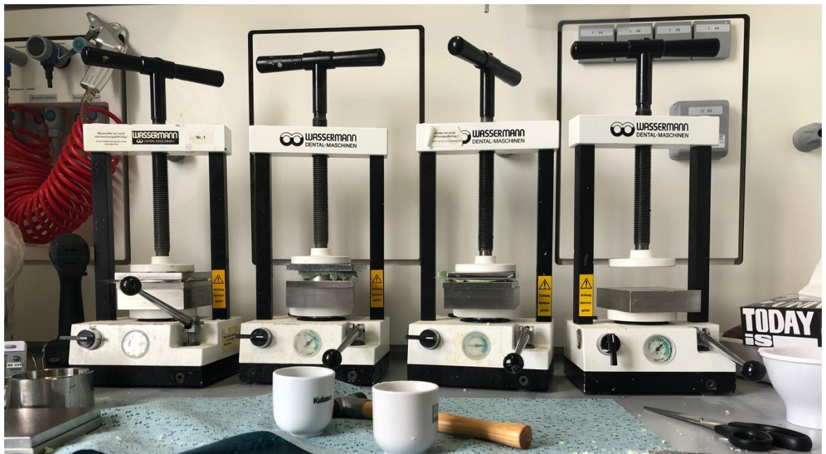
Figure 23: Molds containing cement in the hydraulic presses at 3 bars for 30 minutes
