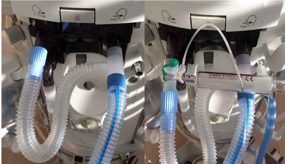
Figure 2: Equipment to sample breath air during anesthesia. The panel on the right shows the glass syringe coupled to the three-way valve
