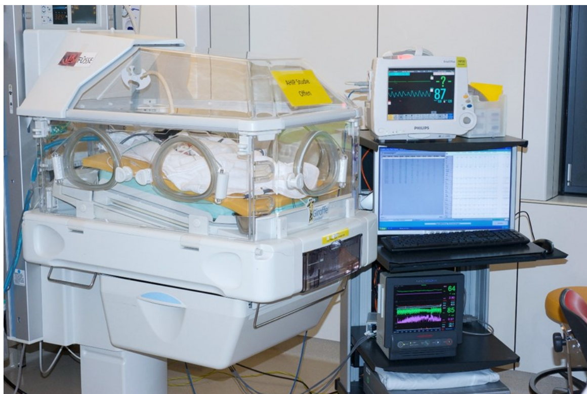
Figure 3: Measuring station with 'Giraffe' incubator (GE Healthcare, United Kingdom), IntelliVue MP50 monitor, polygraphic system, NIRO-200NX.
