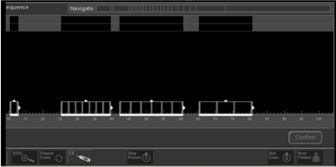
Figure 3. Perfusion protocol with volume scanning distribution in seconds and scan intervals. At beginning two pre-contrast volumes, thereafter eight volumes with 1 s intervals, followed by seven volume acquisitions with a scan interval of 2 s and by further four volume acquisitions with a scan interval of 4 s were obtained.
