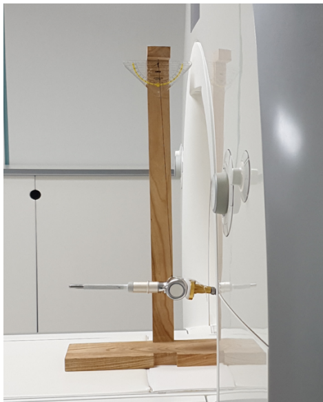
Fig. 14 Tumor Endoprosthesis (MUTARS) with displacement angle of 4°. Slow and moderate alignment with the magnetic field lines observed
