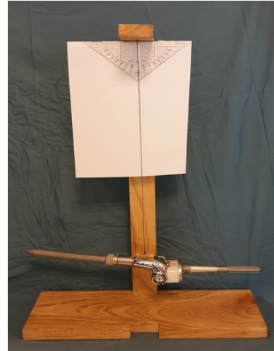
Fig. 7 Displacement Force Fixture with Tumor Endoprosthesis (GMRS) in Testing Configuration
