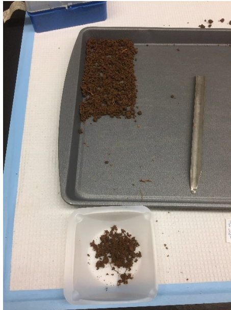
Figure 10. Secondary 2D Japanese slabcake after thirty cores have been taken. The plastic weigh boat contains the soil from the cores.
