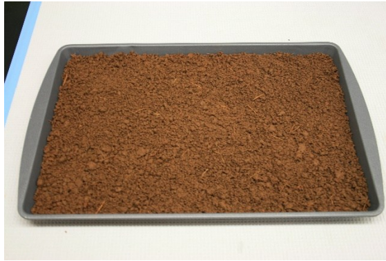
Figure 8. Composite sample prepared for 2D-Japanese slabcake, before cores are taken. Though there is still some degree of irregularity in size, the largest aggregates are smaller than those depicted in Fig. 7.
