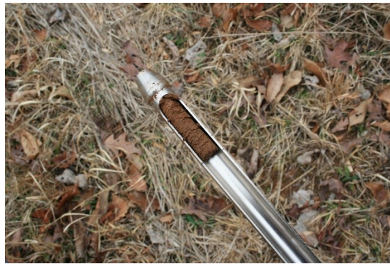
Figure 5. Step probe with core. The taper at the cutting end of the probe assists both with pushing into the soil and with retaining the core inside the probe as the probe is withdrawn.
