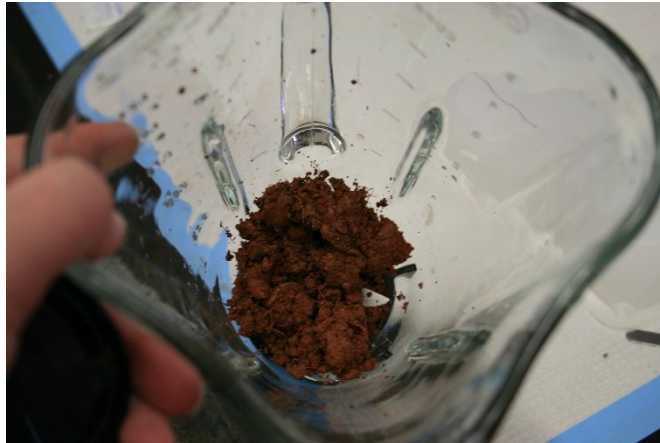
Figure 7. Soil in the blender, demonstrating proper coverage of blade assembly. The soil is depicted prior to any pulsing; the aggregates are irregular in size.
