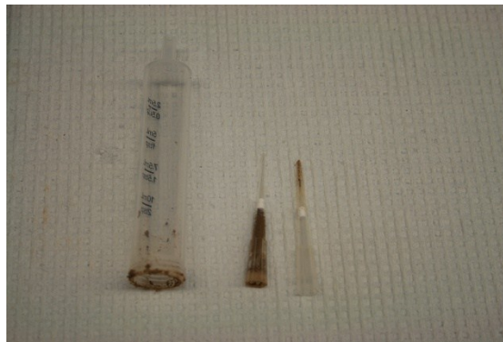
Figure 9. Coring implements: an infant dosing syringe and pipette tips. Soil tended to get stuck in the pipette tip used to take the cores (center), so a second pipette tip (right) was used to remove soil from the coring tip.
