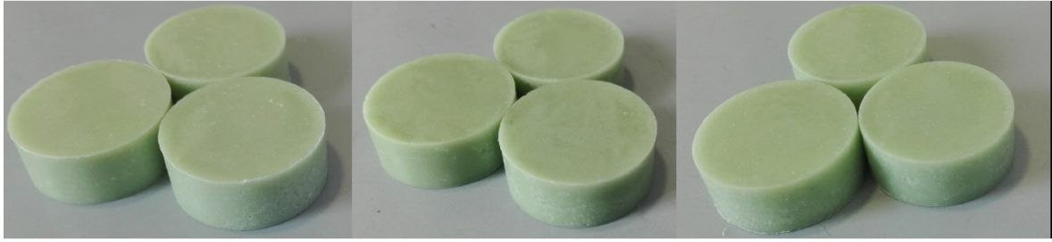
Figure 32: Cement bodies for microbiologic assessments. Panel A: Palacos® R+G with 3 g ampicillin. Panel B: Palacos® R+G with 3 g cefuroxime. Panel C: Palacos® R+G with 4 g piperacillin/0.5 g tazobactam.
