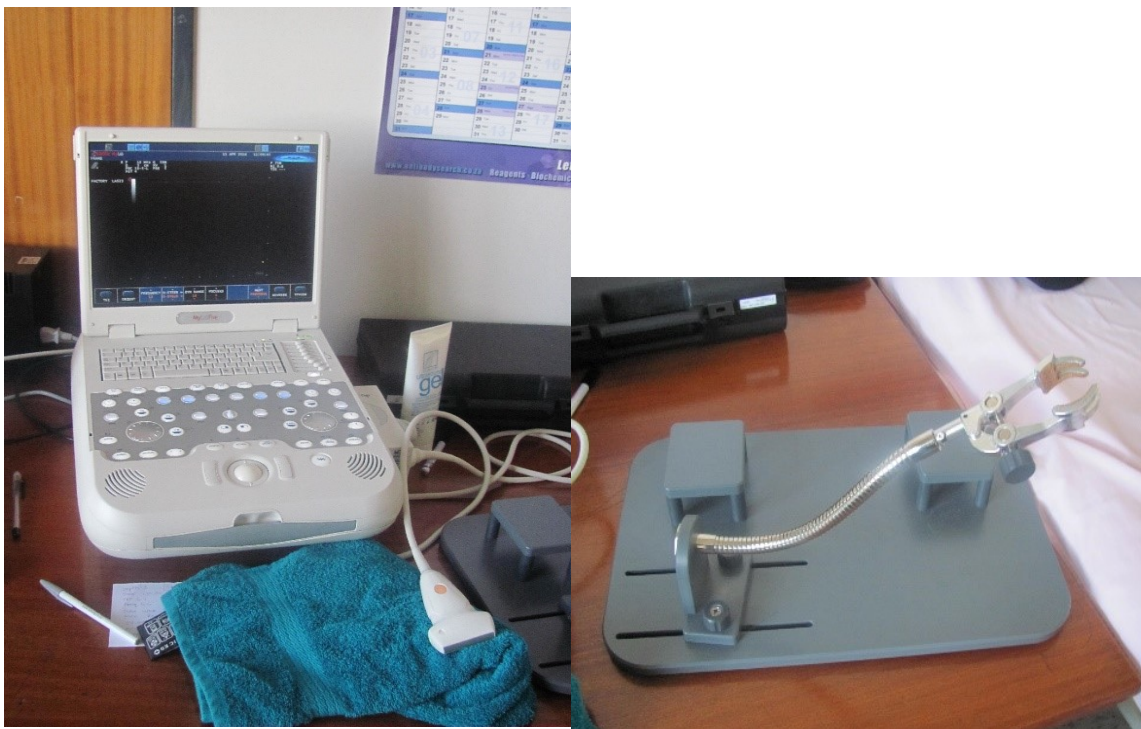
Figure 16: Ultrasound system with ultrasound probe (left) and an ultrasound probe holder device (right)
