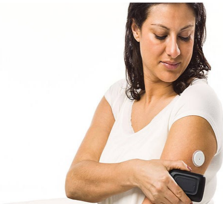
Fig. 22 From Abbott® recommended placement of Abbott FreeStyle Libre® sensor unit on the upper arm. The reader uses near field communication. To show glucose trend arrow, data are transmitted when reader is brought to the sensor. (9)
