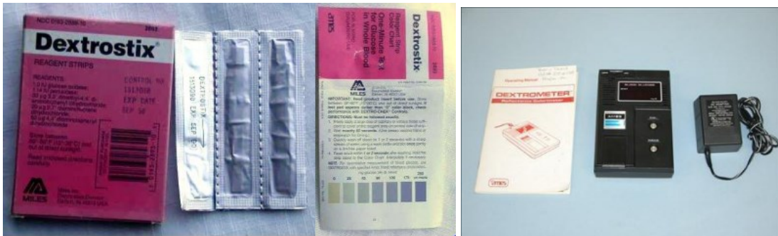
Fig.13 Dextrostix ® urinary glucose strips working on the basis of color change (left panel).Dextrometer ® electronic device to analyze Dextrostix (right panel).(8)
