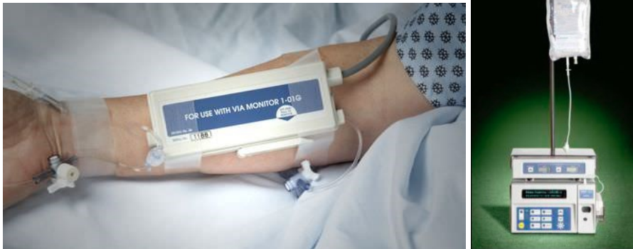
Fig.18 The GlucoScout® accesses blood from a peripheral vein, using glucose oxidase for determination. It first samples about 1 mL of blood and after electrochemical analysis, it returns the collected sample with a non-heparinized calibration solution. (72)
