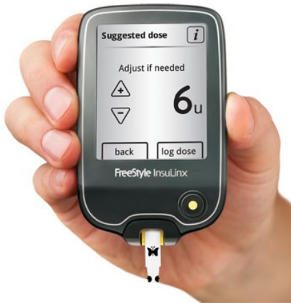
Fig.14 Example of a blood glucose meter (Abbott FreeStyle InsuLinx, Abbott Diabetes Care) (60)
