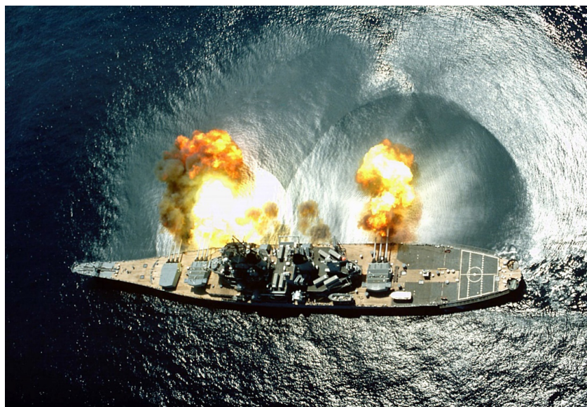
Figure 7 - Illustration of the positive pressure blast effect in water (USS Iowa) Source: (85)
