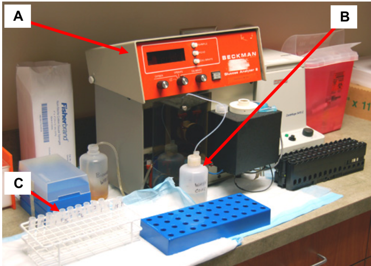
Figure 7 Glucose analyzer: Shown are the Beckman Coulter Glucose Analyzer 2 (A), its reagents for measurement (B) and a holder for the test samples (C).
