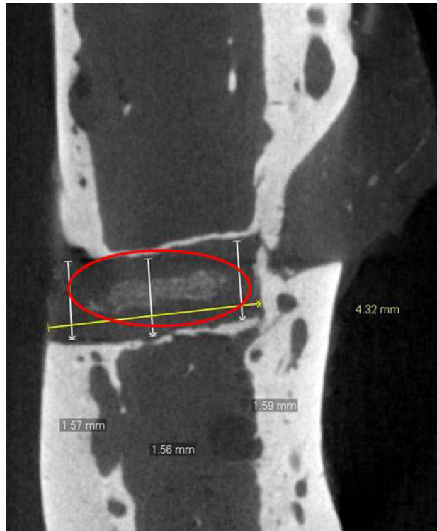
Figure 3.9: High resolution scan of explanted P40Mg implant after 9 months with measured diameter and length of implant
