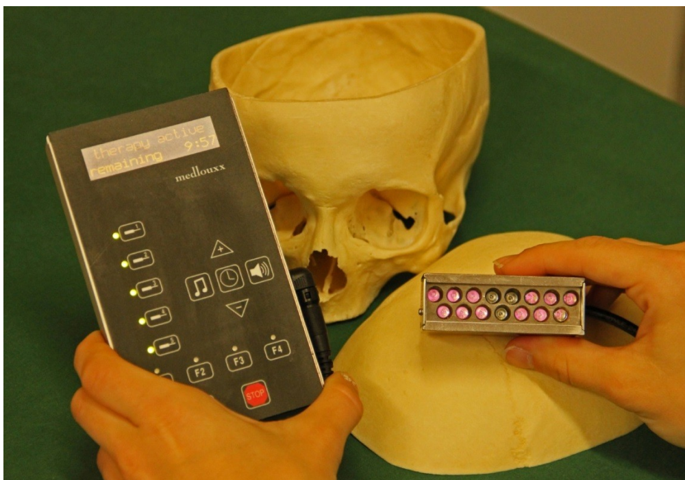
Fig. 3.3: The medloux system including the LED applicator.
