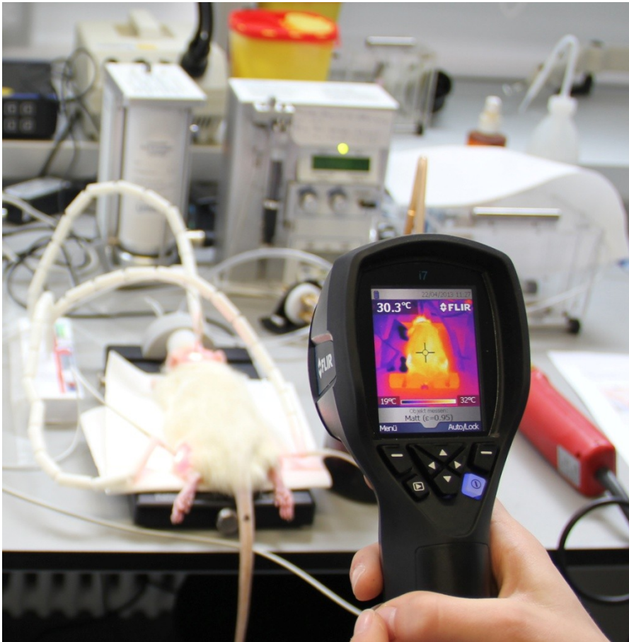
Fig. 4.3: Temperature measurements using a Flir i7 infrared thermocamera.
