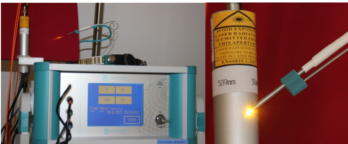
Fig. 2.2: First yellow laser (589 nm, 50 mW) for future medical applications at the Medical University of Graz.
