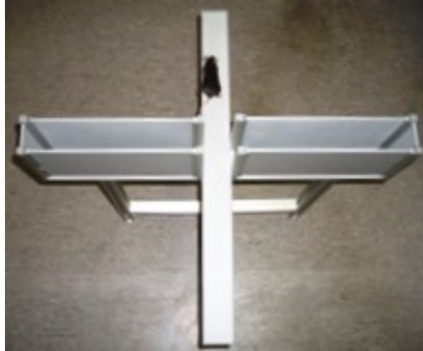
Figure 4 Top down view on the EPM with mouse exploring the open arm
