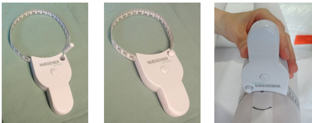
Figure 9: Waegener circumferential tape measure
