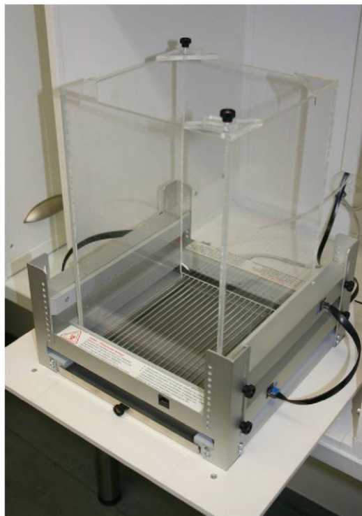
Figure 5.2: Automated box provided by TSE-Systems for the Contextual fear conditioning task.
