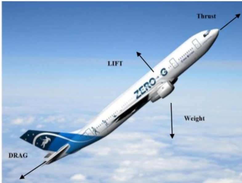
Figure 28: Forces acting on aircraft. Illustration adapted from 'The dynamics of parabolic flight: flight characteristics and passenger percepts.' (Karmali & Shelhammer 2008, p. 14)
