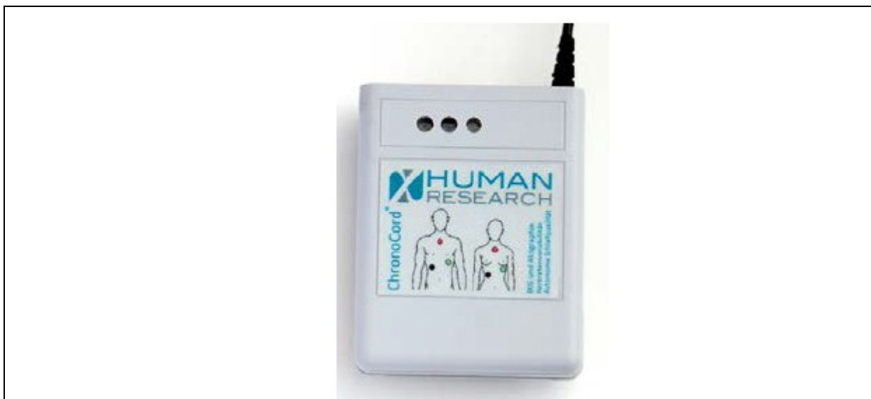
Figure 10: ChronoChord records heart rate and respiratory correlated parameters over 24-hours with a high standard of RR identification
