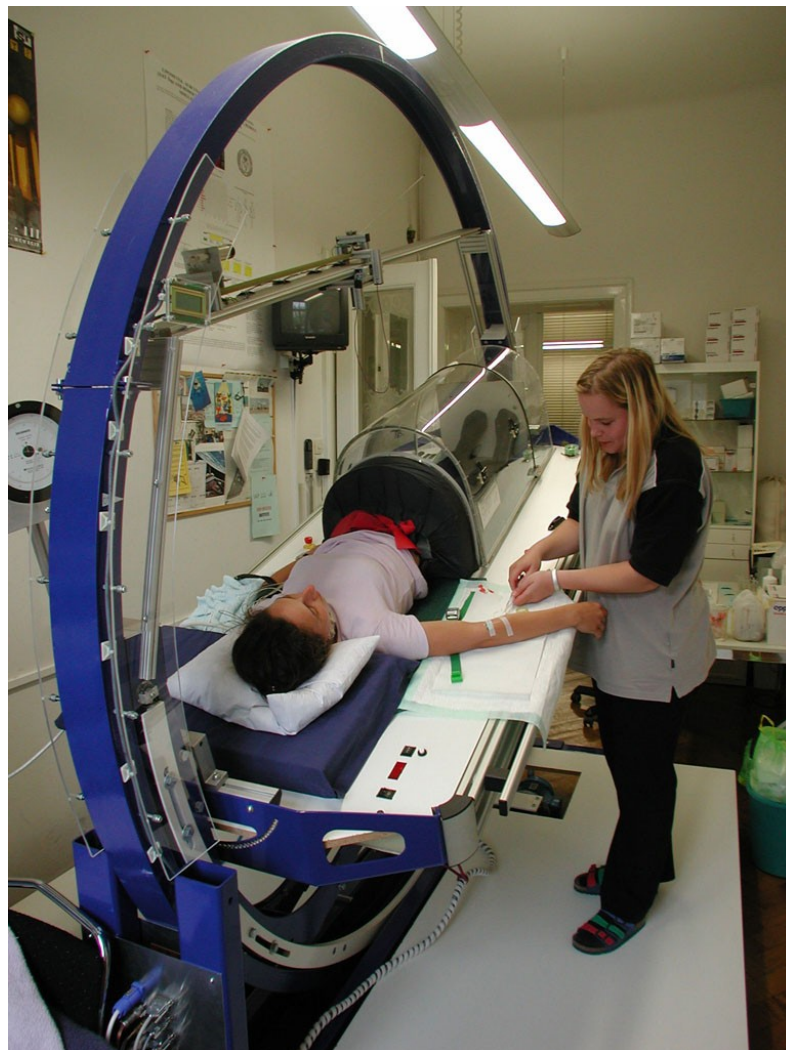
Abb. 3 Automated Human Multi-Stimulation Test Device mit Versuchsperson in head down-Position 42
