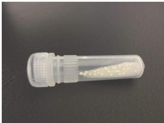
Fig. 3.7: Vial containing ceramic beads.
