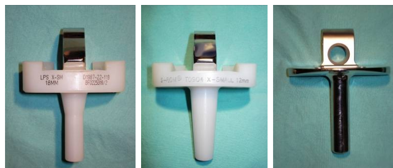
Fig.13: The tested PE-inlays/stems: LPS™/M.B.T., S-ROM Noiles and GMRS™.
