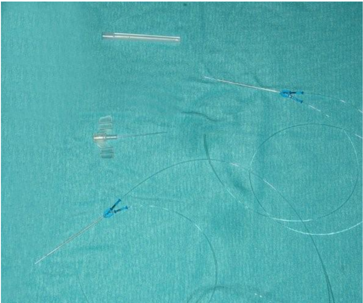
Fig. 24 A microdialysis probe with two interleaved and stucked together cannulas, the thinner and internal probe is a little bit longer. At the tip of the probe is a semipermeable membrane, which is fused to the external probe. The probe's inflow tubing is connected to a microperfusion pump and so the probe is constantly perfused with a physiological solution. Samples are continuously collected from the outflow tubing. 105 106
