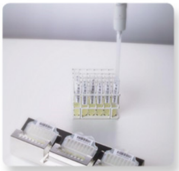
Figure 21. Loading of the samples into the 8-well sample vessels.
