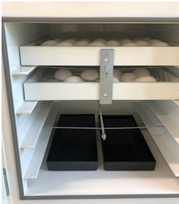
Figure 6. Horizontal placement of the eggs on the brood roll hordes in the incubator. The brood roll hordes were fixated with a metal plate to ensure slight movement of the eggs. The black water tanks can be seen below.
