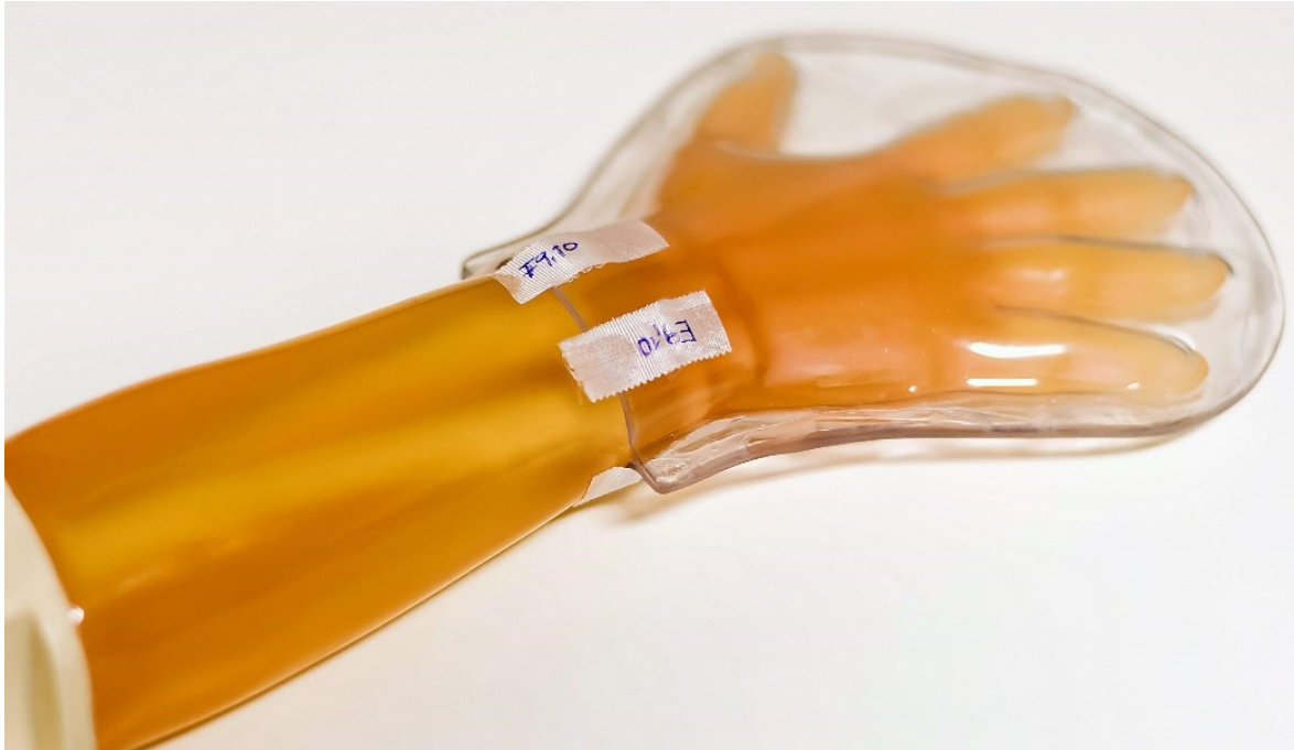
Figure 7. TLDs attached in clockwise positions around the pediatric wrist phantom. Before the start of every measurement, we manually taped the dosimeters to the phantoms as depicted in the image above.
