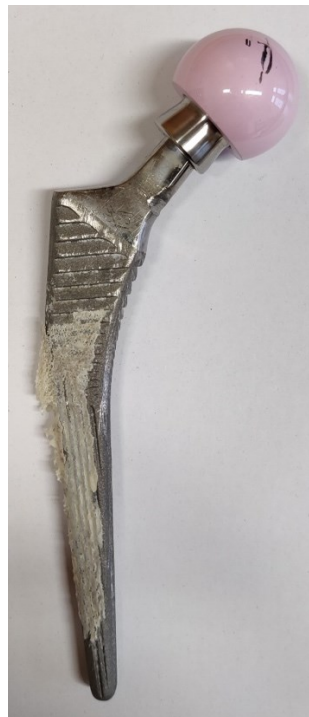
Figure 2. Explanted UHNA with a Lateralized Configuration and Ceramic Head.
