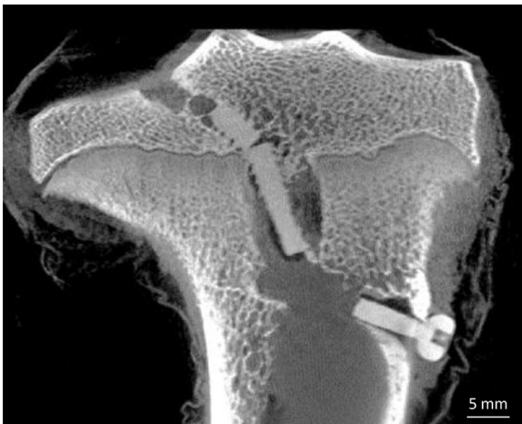
Fig. 12. Broken screw in the 12-weeks group with transepiphyseal position.
