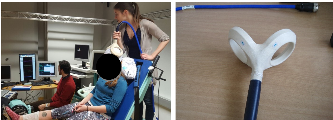
Figure 19: left: Volunteer sitting in the dynamometer chair with the foot on the footplate during TMS measurement. right: coil.
