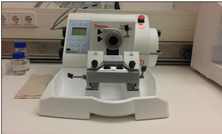
Figure 2.2: Rotation microtome used for cutting Technovit 9100 New embedded bone samples.
