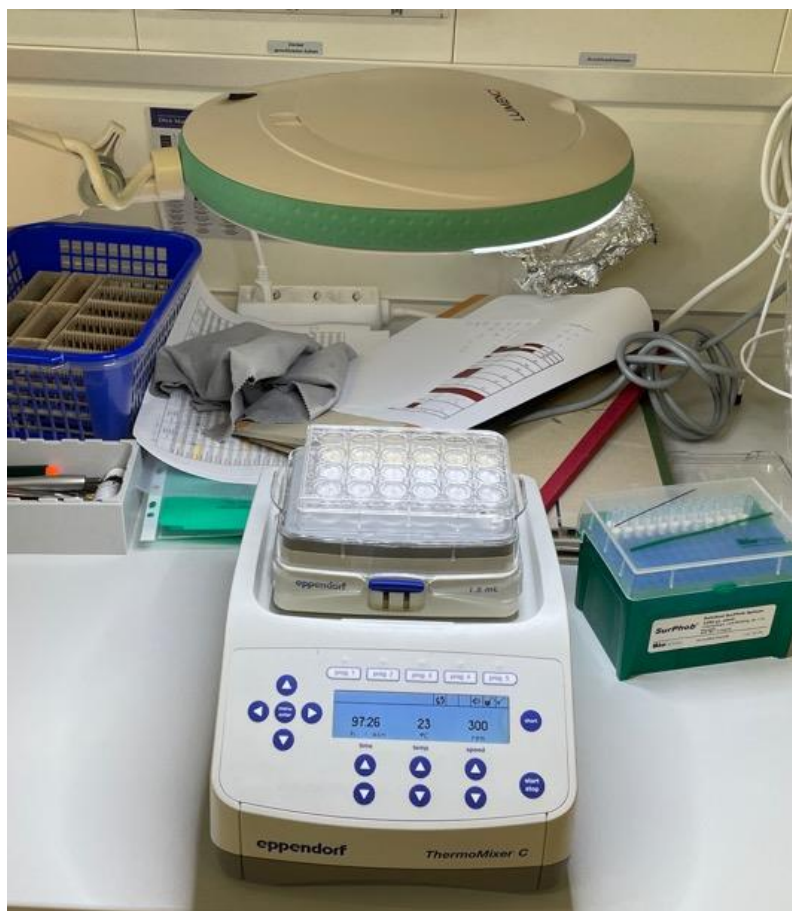
Figure 5 Experimental setup for the measurement of ROS production under constant light exposure. The NP suspensions were incubated in a 24-well microtiter plate for 1 h at room temperature under constant shaking (300 min -1 ).
