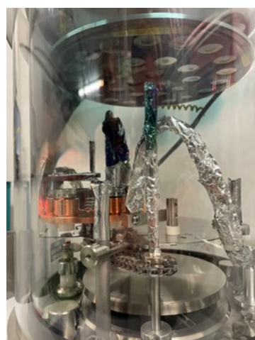
Figure 29 PVD chamber for the deposition of organic pigments. PVD chamber and schematic representation with the rotating mask holder and the inlet for the glass coverslips, quartz crystal for measuring the deposited pigment thickness, crucibles for heating up the pigments and a shutter.
