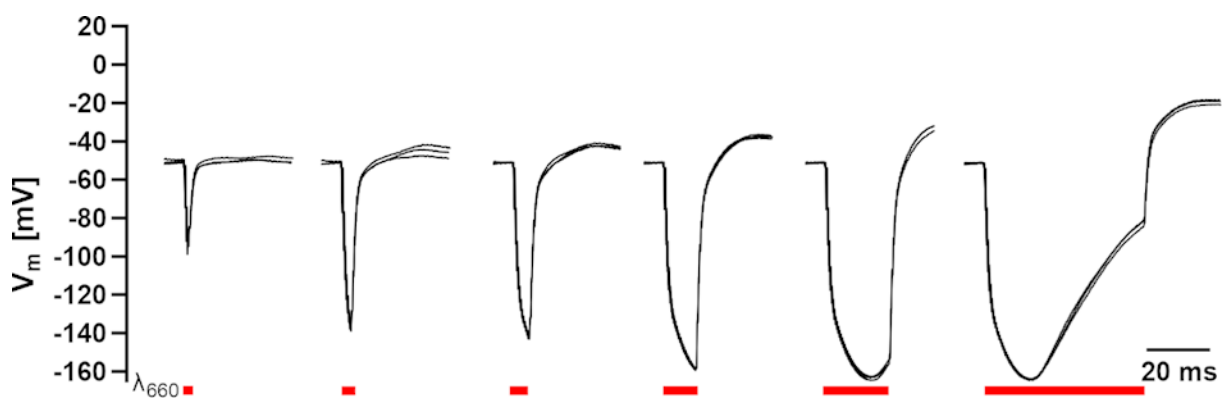
Figure 74 Light pulse length comparison and the cathodic stimulation artifact in current clamp. Zoom into the different light pulse lengths and a representative time course of the recorded potential of generally nonresponsive neurons. Overlay of three recordings of a cell on PEDOT:PSS spin-coated OEPCs in a gap free mode. Adapted and reproduced with permission from John Wiley and Sons: Advanced Materials Technologies, [20], under the terms of the Creative Commons CC BY license.
