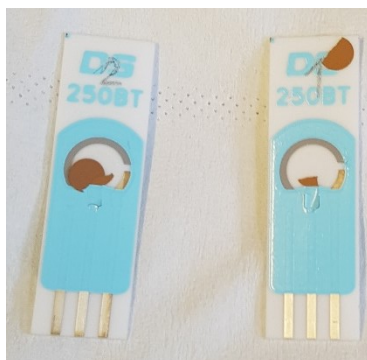
Figure 27 : BT electrodes were destroyed by too harsh cleaning.
