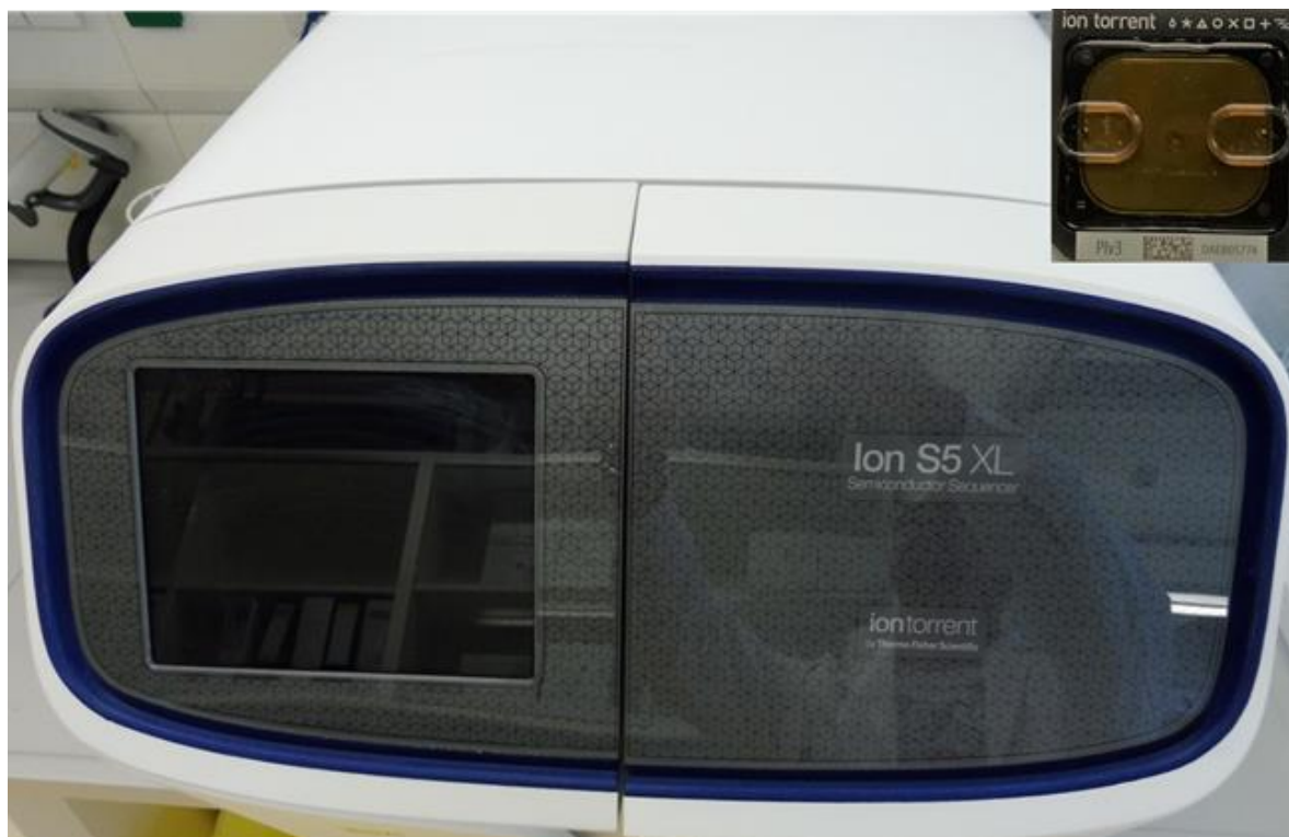
Figure 7: Transcriptome Sequencing by Ion Torrent Next-Generation Sequencing. Automated production of Ion AmpliSeq transcriptome libraries using the Ion S5 XL and Ion P1v3 Chip containing 8 barcoded chips for sample tracking.
