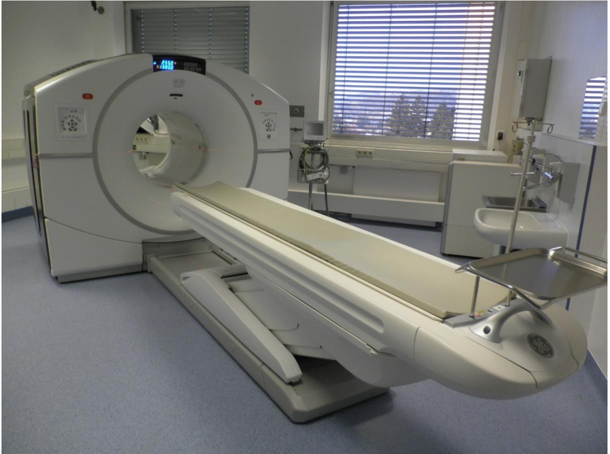
Figure 7: Discovery MI Gen 2 (GE Healthcare, Chicago, Illinois, U.S.A.) PET/CT device.
