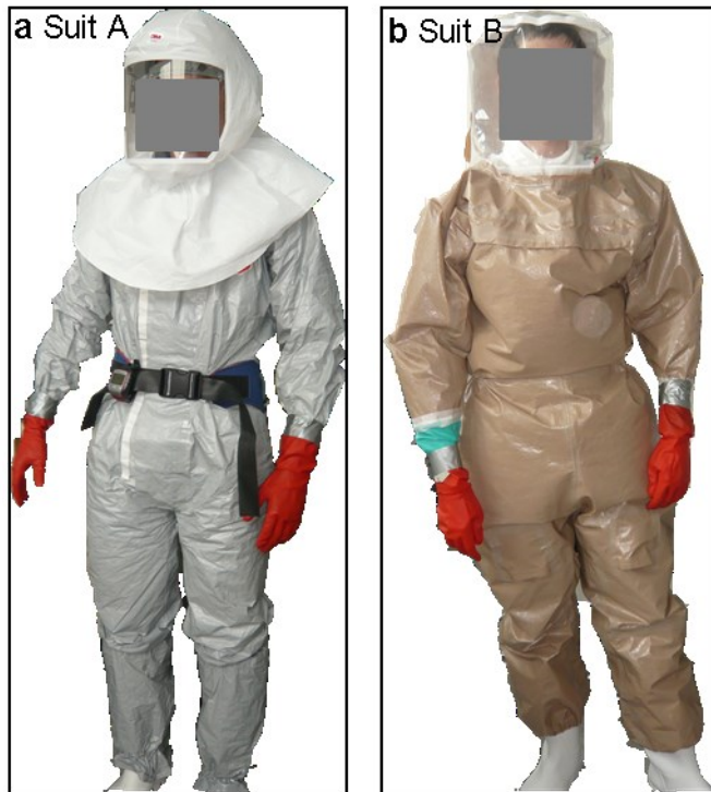
Figure 6: Two different PPE types used for the study. Suits tested vary in their respiration system and face shields. a: Suit A, head ventilation with external fixation of the air filters on a belt. b: suit B, total suit ventilation with internal respiration system worn on a rucksack inside the suit (Loibner et al., 2018).
