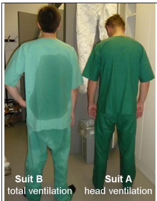
Figure 9: Fluid loss illustrated by sweat soaked undergarment. After termination of all four series at 28 °C the fluid loss was visible by the differently sweat soaked undergarment. The left subject was allocated to suit B, the right subject to suit A.
