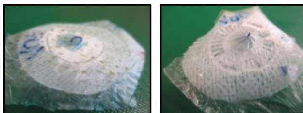
Figure 25: Examples of catheters that kinked above adhesive and did not insert into the skin.
