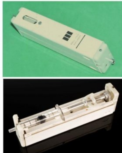
Figure 2: The "Mill Hill Infuser" (top) and with the casing removed (bottom) showing the syringe drive [5].
