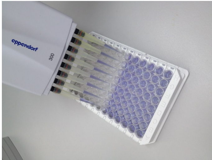
Figure 15, showing the 90 well plate being filled with the blue conjugate solution, which contains the anti-GM monoclonal antibody, which binds to GM antigens on the micro well floor if the sample is positive.
