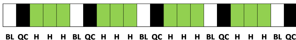
Figure 2: Sample sequence (BL: Blank samples, QC: quality control = pooled samples, H: human serum samples)
