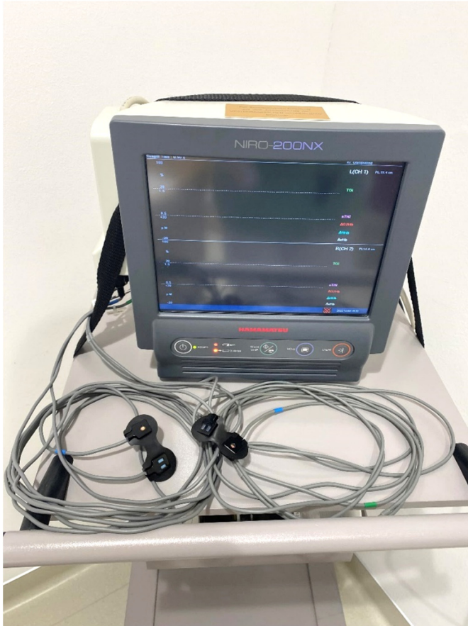
Figure 1. NIRS 200NX (Hamamatsu Photonics K.K., Hamamatsu City, Japan) Near-infrared spectroscopy monitor with two sensors for cerebral and peripheral NIRS measurement.
