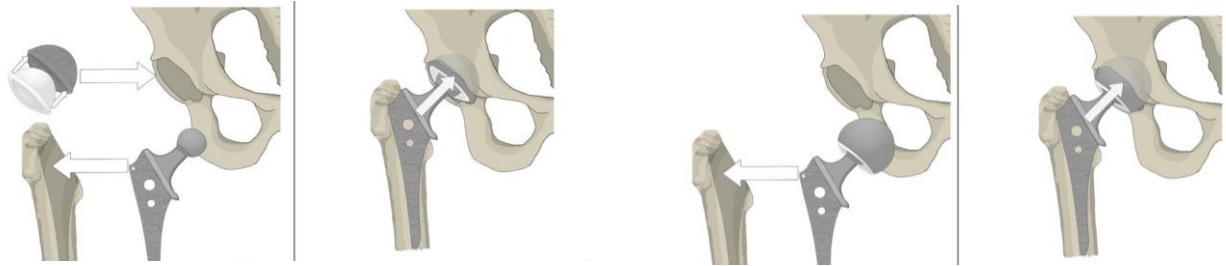
Figure 2 shows the process of implantation of a total hip arthroplasty (THA) on the left versus partial hip arthroplasty on the right.
