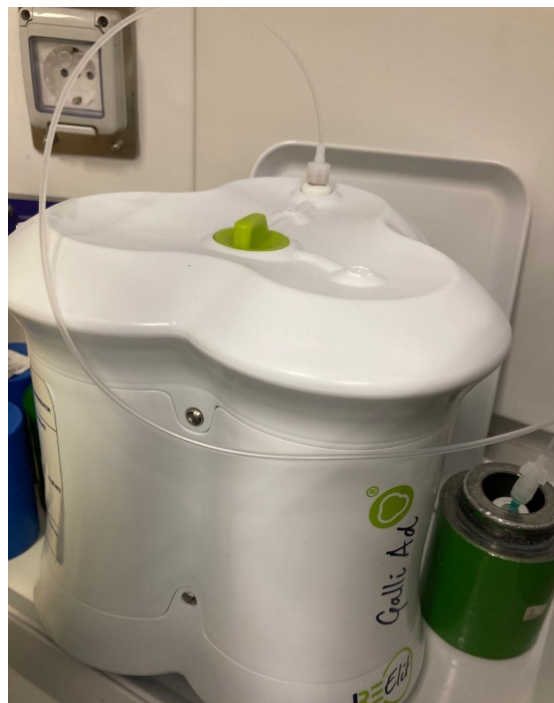
Figure 5: Galli Ad ® generator. Notice the green lead container on the right side; this is where the eluted ^{68}\text{Ga} is stored.
