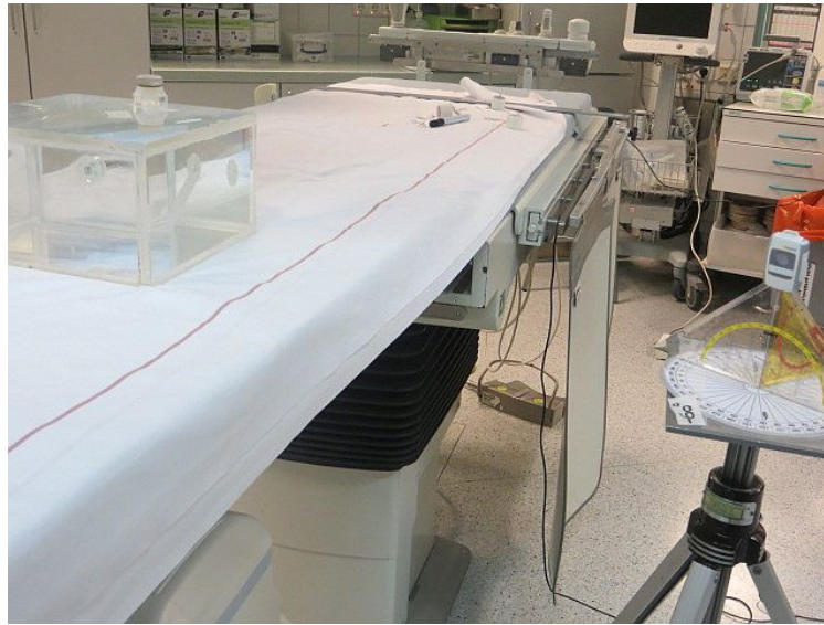
Figure 16: Experimental Setup - Angular response of PDMs in horizontal plane
