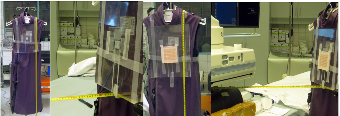
Figure 19: Experimental setup for calibration of TLD 100-H chips
