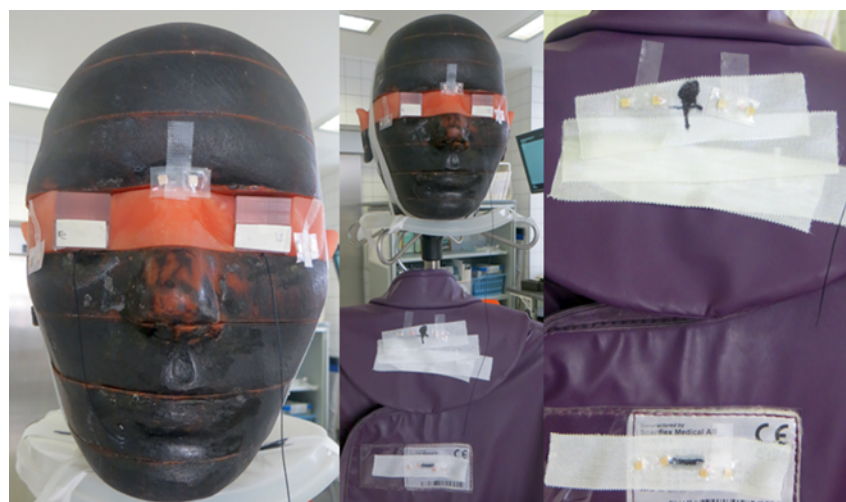
Figure 21: Placement of TLD 100-H chips at reference points
